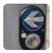
At street corners with lights, pedestrians will find a button with a raised directional arrow making a slow beeping sound. Pushing below the arrow tells the light sequence that a pedestrian wants to cross. There is a symbol of the walking man in green and a fast clacking sound to indicate when it is OK to go. The arrow symbol will vibrate when it is OK to go for people who get their safety information by touch. These buttons are found on tall traffic poles and also on half poles.
